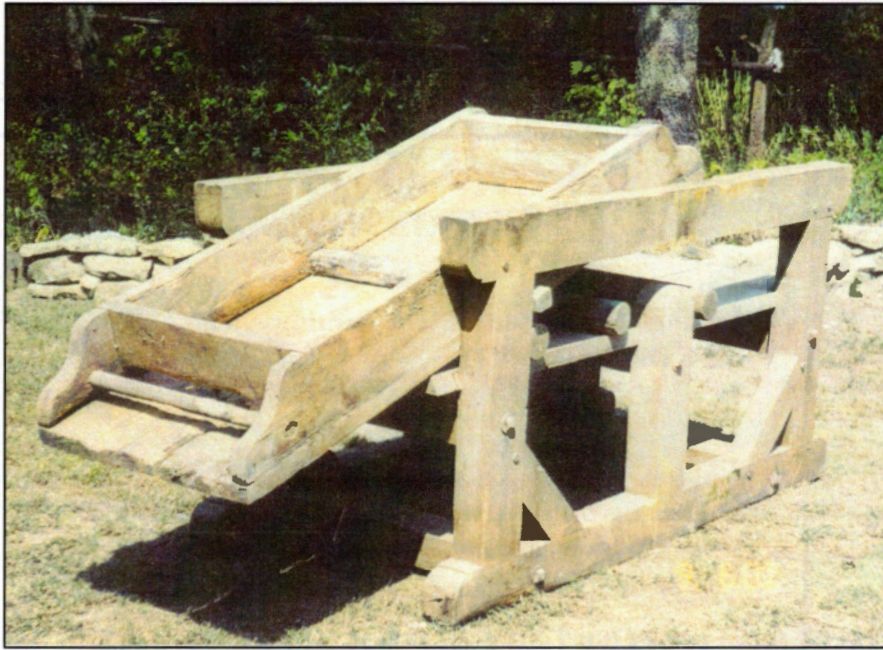
This mangle used to press wet laundry was made by Jacob Harder about 1885. Measurements are 70 inches long, 38 inches high, and 34 inches wide.
